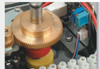
Position Transmitter 12.5VDC to 37VDC, 4-20mA (Excludes APL-2)
