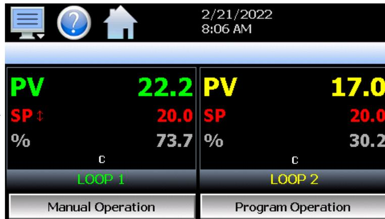
Under ramp rate operation, when a set point is entered, the loop starts the ramp from the current process value and then continues to the target set point according to the rate up or rate down entry made on the set point Limits screen (see section [9.3 Setpoint Limits](#)). The target set point, ramp rate and deviation hold entries can be viewed at any time by pressing the SP tag for the loop.
