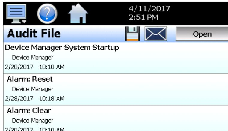
Each action recorded to the file includes the date/time it occurred as well as the user (if logged in) that made the change. If no user is logged in, the user will be listed as “Device Manager”, which is the default user account for the MCT4 system.
