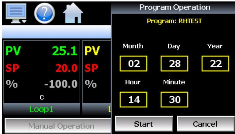
The date and time fields will automatically populate with the current date and time (within the next half-hour increment). Each field can then be set to the specific date and time desired for the program to begin. When the Start button is pressed and a start step entry is required, the Start Step entry will be shown; otherwise, the program will be placed into TOD start from step 1.
