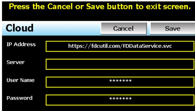
The **IP Address** field is used to enter the IP address of the remote server site that MCT4 is to interface with.
