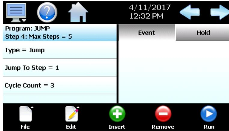
To program a jump step, select jump for the step type and enter the step number that you want the program to jump back to along with the total number of times the jump is to be made (by pressing each row in the list). A cycle count of one indicates that no jump will be made since one cycle is completed upon reaching the jump step.
