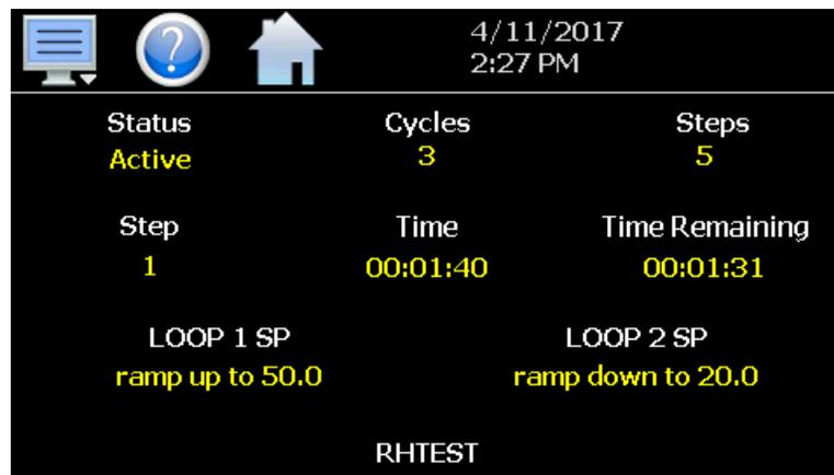
The **Status** field indicates the current operating mode of the program, i.e., On, In Hold and Off.
