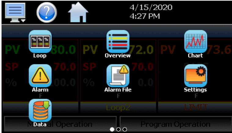
Slide page 1 provides navigation to all standard view screens. These include the Loop and Overview, Chart, Alarm monitor, and Alarm File.
