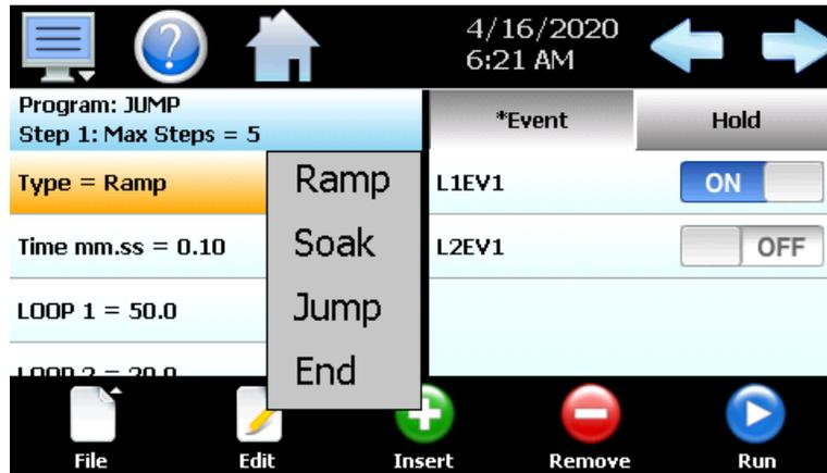
The **Ramp** selection allows the user to program each loop to ramp to a set point in a specific period of time. Simply select ramp from the pop-up menu and then enter the loop set point(s) and time.
