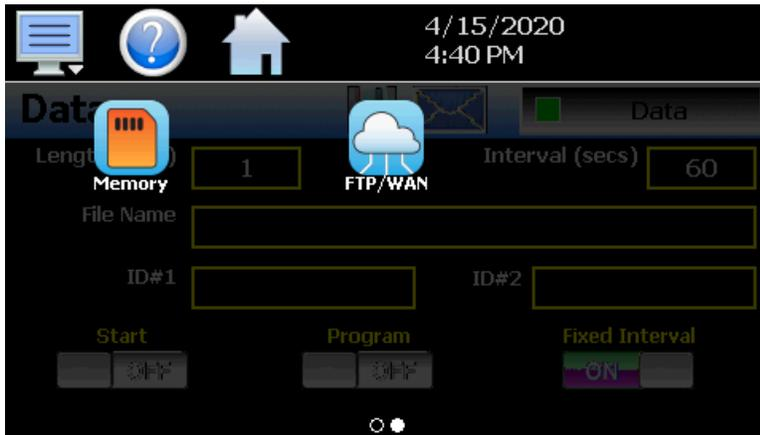
Slide page 2 provides access to the FTP/WAN back-up settings and the memory check utility for viewing available system/storage memory space.
