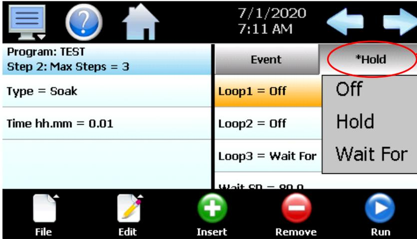
When at least one hold condition set in a step, an asterisk "\*" will appear before the word "Hold" on the list selection button.
