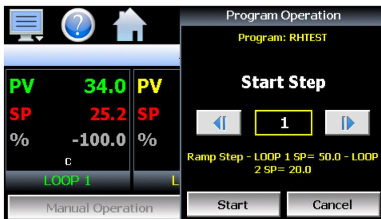
The **start step** can be adjusted up and down by pressing the right/left arrow buttons or by pressing the step number field and directly entering the desired start step via the numeric keypad. Once the desired start step number is entered, press the “Start” button. The program will then be transferred to the loop control(s) and started once the transfer is complete.
