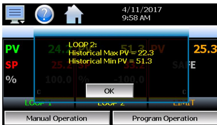
Pressing the “OK” button will close the dialog window and return to the Loop view screen. The historical values are reset each time the runtime application is started and can also be manually cleared by pressing the “PV” tag on the Loop view screen.
