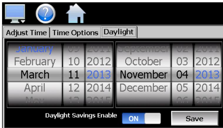
If your locale utilizes daylight savings time, set the start and stop dates for daylight savings and turn on the “Daylight Savings Enable” option. Press the “Save” button to store the settings. MCT4 will then automatically update its clock for daylight savings time.
