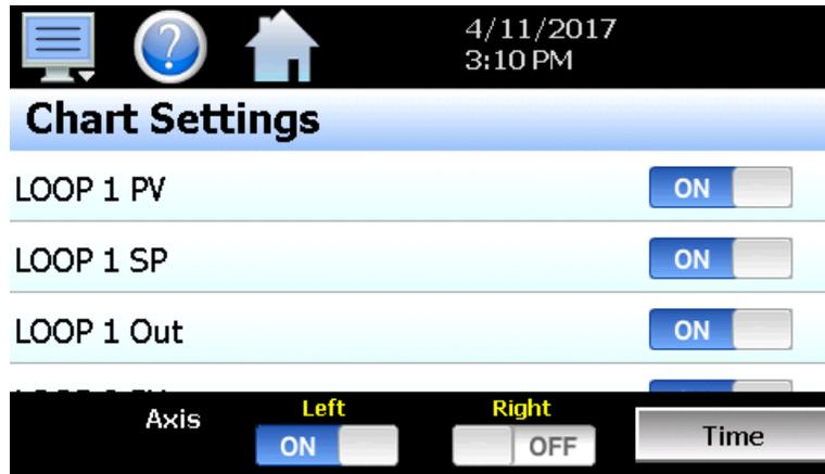
Any point from the data file can be selected along with the vertical axis to be used for each channel to be plotted. Select channels from the list by turning them on or off and use the “Left” and “Right” axis buttons to assign the selected item to the left or right axis for the plot range. To adjust the period of time to plot from the data file, press the “Time” button.
