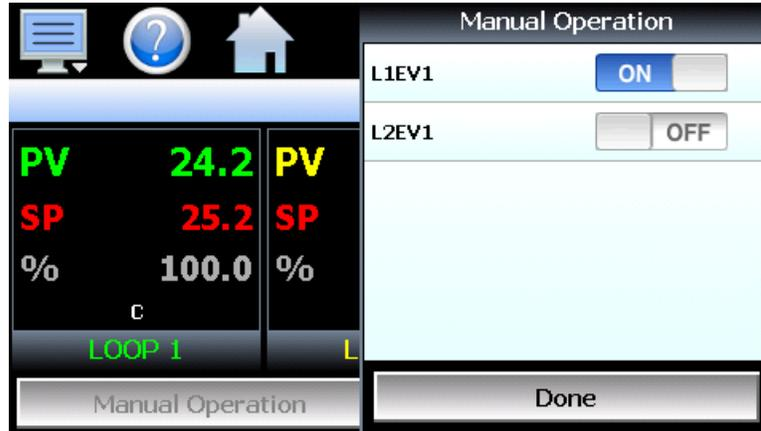
**NOTE:** The MCT4 loop controls can provide up to 3 event outputs each (for a total of 9 events). Depending upon the configuration of MCT4, some outputs may perform specific control or alarm functions. The use of each output, and what it controls, is determined by the system designer. If there are questions or concerns about the configuration and operation of your MCT4 controller, contact your OEM for further information. Only your OEM can address equipment related issues.
