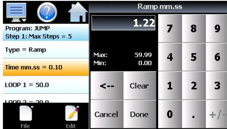
**NOTE:** A step time of zero can be entered for a step to implement an immediate set point change when programmed for ramp. If holdback is enabled on a step, a minimum step time of 10 seconds 0.10 (mm:ss) or 1 minute 0.01 (hh:mm) is required to ensure that the holdback condition can recognize the process change in order for holdback to operate.
