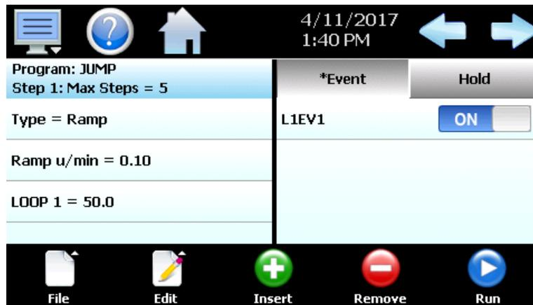
**NOTE:** A ramp rate entry is only available for single loop MCT4 systems because the length of time for the step to complete is based upon the change in set point and the rate at which the set point is to ramp. Ramp units of time are still available for selection on single loop systems if time entry is preferred over rate.
