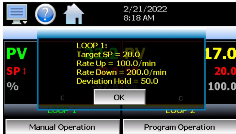
Pressing the “OK” button will close the dialog window and return to the Loop view screen. The Overview screen indicates a loop under ramp conditions by displaying the target set point in parenthesis after the actual loop set point.
