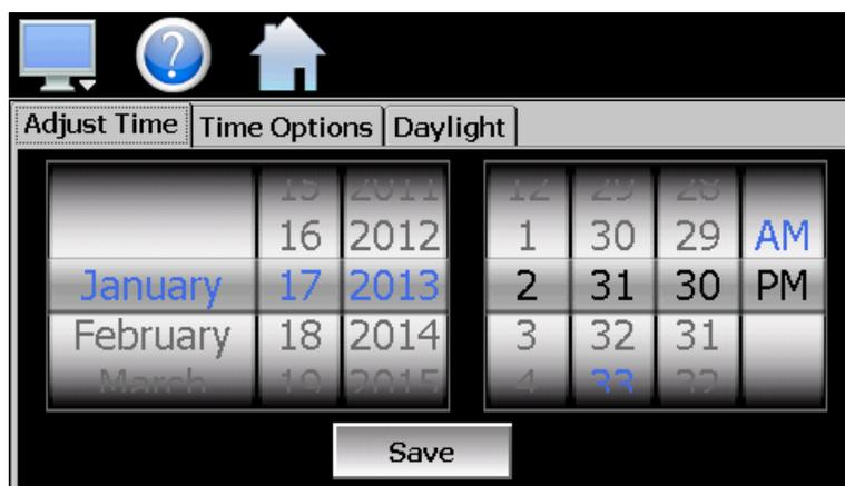
To make adjustments, scroll each time wheel to adjust the month, day, year, hour, minutes, seconds and AM/PM selection. Once all adjustments have been made, press the “Save” button to set the system clock to the date and time entered.
