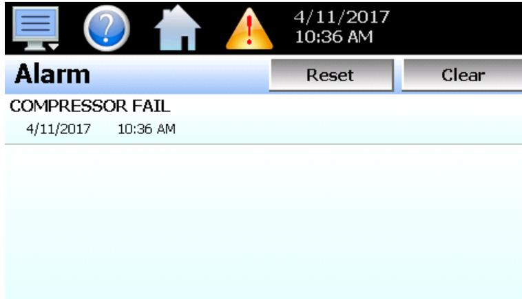
The alarm will be removed from the list when cleared by the operator by pressing the “Clear” button. Only alarms that are not currently active in the system can be cleared from the alarm list.
