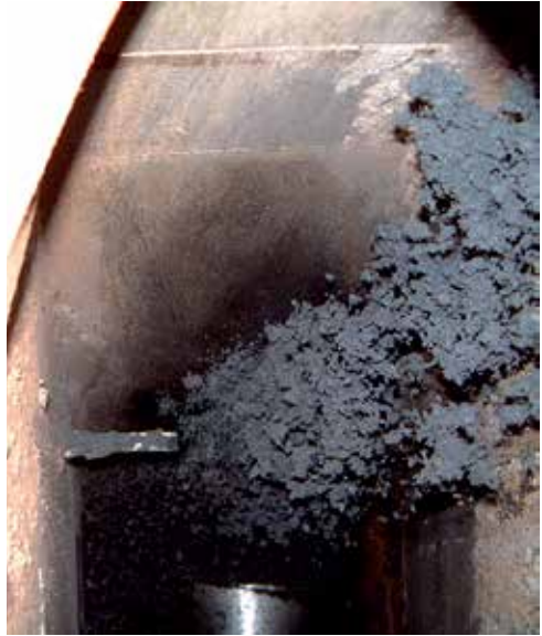
Continuous filling with build-up on probe
