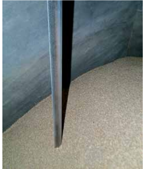
High level switch in plastic pellet silo
